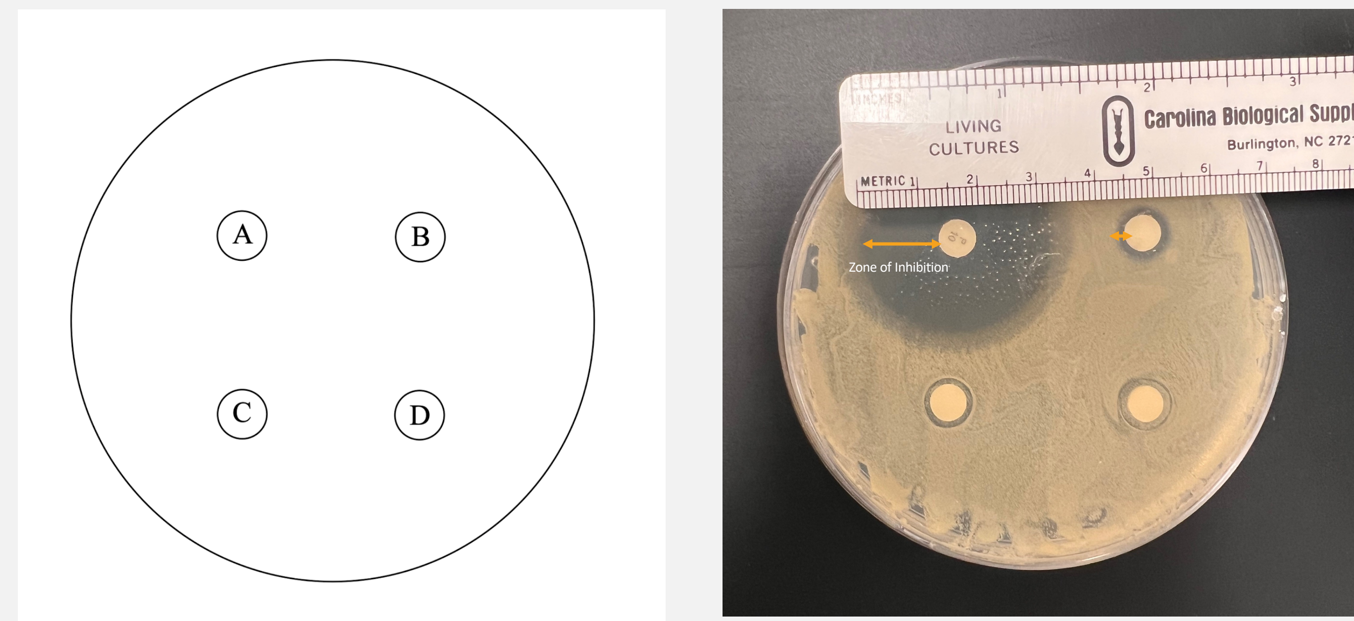
Figure 1. Mueller Hinton Agar plate arrangement with 4 disks, A-D, of different treatments for S. aureus . Disk A contains 10 \mu g penicillin, Disk B contains 1035 ppm calcium hypochlorite, Disk C contains a morning pool water sample, & Disk D contains an evening pool water sample. Also pictured is a Mueller Hinton Agar plate following completion of the Kirby Bauer Assay, showing measurements of the zones of inhibition in millimeters.
